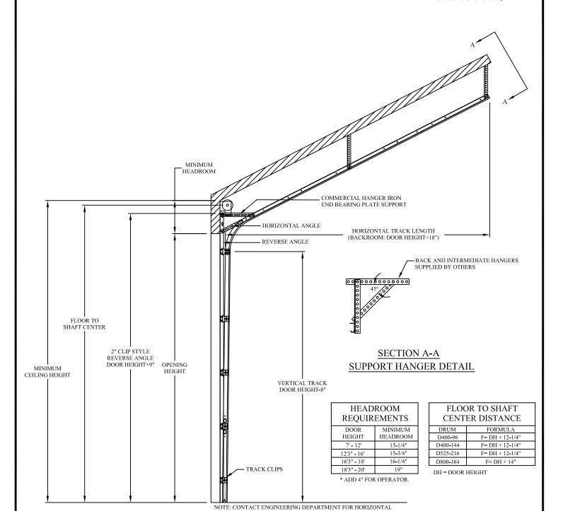
STANDARD LIFT FOLLOW THE ROOF PITCH ANGLE MOUNT TRACK SET DETAIL
